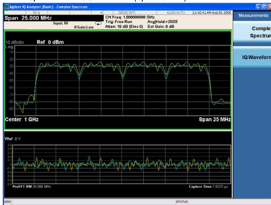
Spectrum and I/Q Waveform (Span 25 MHz)
