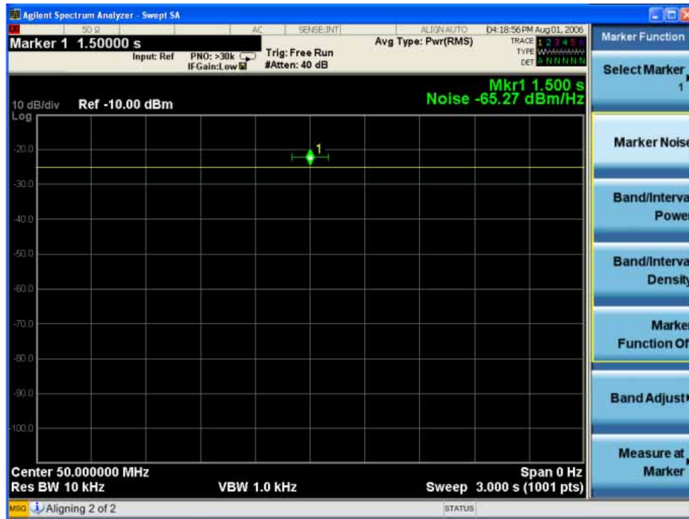
Figure 7-3 Noise Marker with Zero Span
