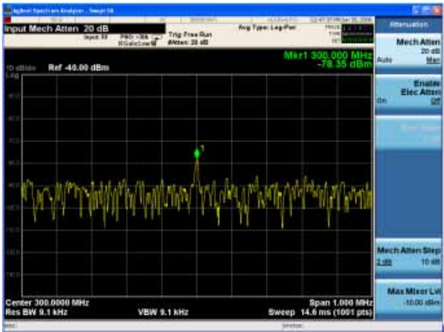
Figure 3-1 Measuring a Low-Level Signal Using Mechanical Attenuation
