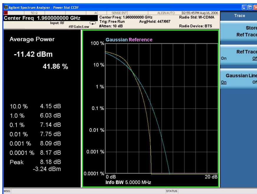
Figure 9-6 Power Statistics CCDF Measurement on a W-CDMA Signal
